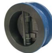
Art. 2401 Wafer type. Double disk check valve PN 16 DN 50-300
